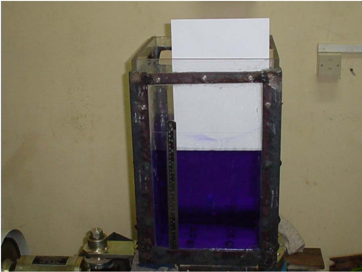
Figure 8.7 Method for measuring the water surface profile at resonance; notice the blue trace left on the white paper by the oscillating liquid surface.
