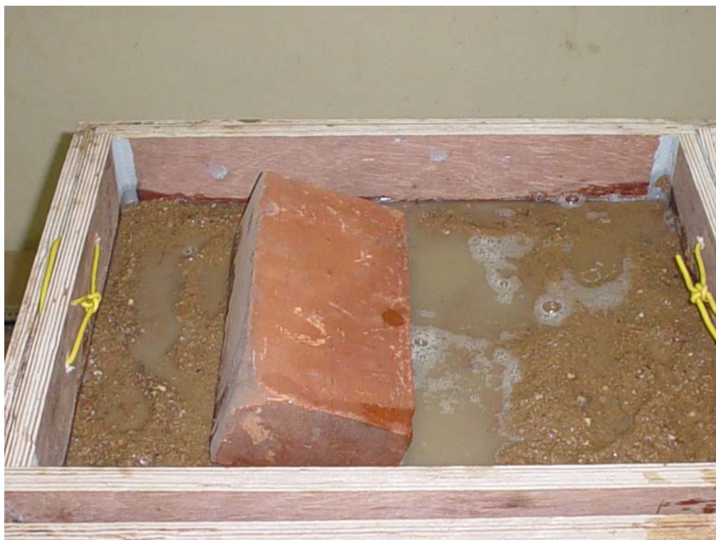
Figure 10.10 The state of the brick block after liquefaction has occurred; notice the ponding of water at the surface. Figure 10.4a shows the state of the system before the dynamic base motions are applied.
