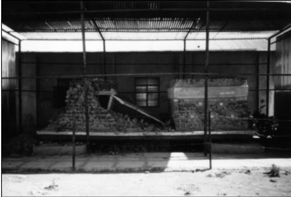
Figure 35 Experimental verification of the retrofitting technology at Umarga, Osmanabad district. A retrofitted model is shown at the right and the unstrengthened model (damaged) is shown on the left.
